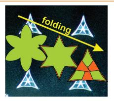
Highly complex multi-step folding of isotropic stimuli-responsive polymer bilayers results in a variety of 2D and 3D structures. Experimental observations allow determination of empirical rules, which can be used to direct the folding of polymer films in a predictable manner.
