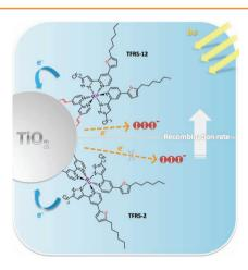
A new class of thiocyanate-free Ru(II) sensitizers with 4,4'-dicarboxyvinyl-2,2'bipyridine anchors are synthesized and used in dye-sensitized solar cells (DSCs). The DSCs are investigated via currentvoltage characteristics, incident photonto-current conversion efficiency (IPCE), impedance spectra, as well as transient photocurrent and photovoltage decay measurements.
