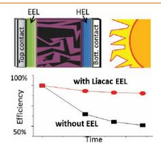
Exposure of organic solar cells (OSCs) to light results in degradation in all OSC parameters, even in inert environments. The use of electron extraction layers (EELs) in between the organic layer and an Al layer can largely suppress contact photo-degradation and enhance OSC photo-stability. Lithium acetylacetonate, as a new EEL material, provides efficiency improvement on par with the ubiquitous LiF, but with some additional stability improvement.
