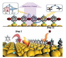
A possible way to fabricate a half-metallic sandwich molecular wire on a silicon surface is proposed using first-principle calculations. The magnetic state of this molecular wire is sensitive to the electric field and can be changed between two states. The hybrid system has very promising application in emerging molecular electronic or spintronic devices.
